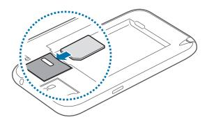
3 Push the SIM or USIM card into the slot until it locks in place.
