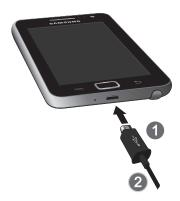
**2.** When charging is finished, remove the flat end from the interface connector jack on the phone.
