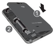
2. Press along the edge of the back cover (3) until you have a secure seal.
