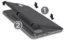
2. Press along the edge of the back cover (3) until you have a secure seal.
